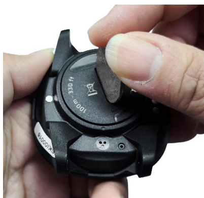
Rotating the battery cover
