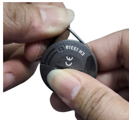
Removing the old O-ring
