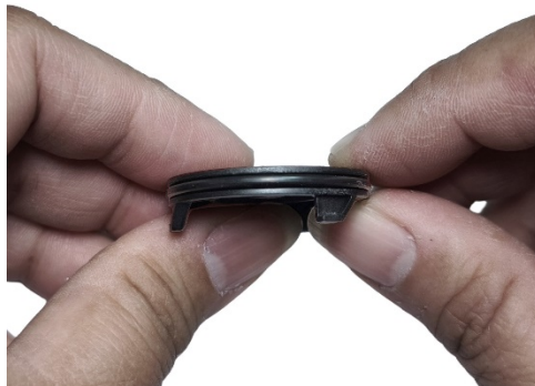
Replacing the O-ring
