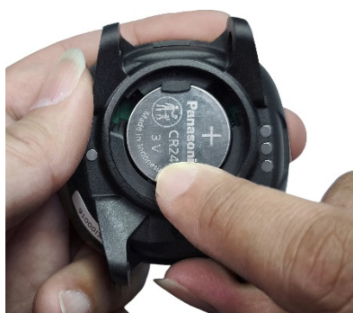
Installing the new battery
