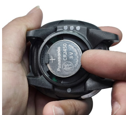
Removing the old battery
