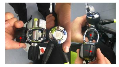
For Oceanpro DIN configurations, slowly turn the DIN wheel counter clockwise and remove from inside the cylinder valve. Immediately dry and replace the inlet dust cap back into a fixed position, to eliminate any change of water entry into the first stage. Note that soaking of your regulator in clean fresh water for a minimum of 30 minutes is now possible.
