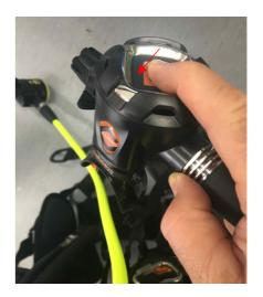
Perform a physical inflation / deflation test of any accessories connected to the regulator to, such as your BCD inflator, to ensure full and complete operation of the SCUBA system.
