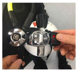
Secure the regulator to tank valve firmly by hand only, whilst holding the regulator in-line and in position with the other. Once secure slowly open valve to prime the regulator with gas, listening for any sign of air leakage.
