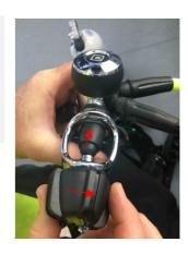
Temporarily pull back hose protectors, run a gentle stream of water over the hoses along with the first and second stages to get rid of any remaining particles that may be trapped throughout any areas of the regulator.
